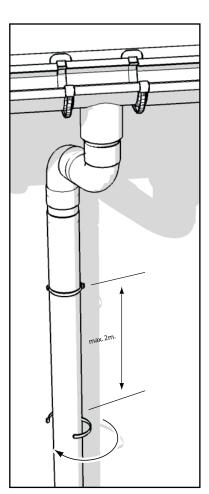
Fix the pipe brackets at a maximum of 2 meters.
