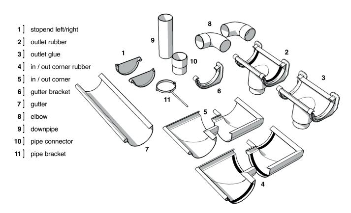
Determine the position of the outlet. That is automatically the lowest point. After that, you can also determine the highest point. Install a bracket at the lowest and one at the highest point. A string secured between both brackets will assist in installing the remaining hangers.
